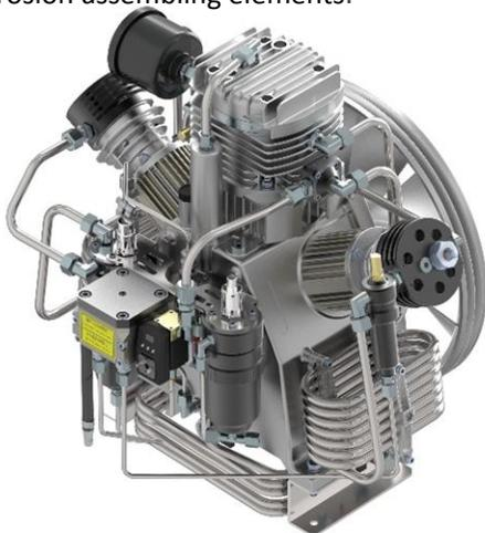
The bearings of the crankshaft have rollers, extremely robust and made in Europe which guarantee a long life of the compressor. An oil pump provides a constant lubrication of the inner workings of the block with oil cleaned of impurities by a filter and by a magnet which catches any metals present in the lubricating oil. The compressed air cooling is obtained by inter-stage stainless steel cooling coils.
